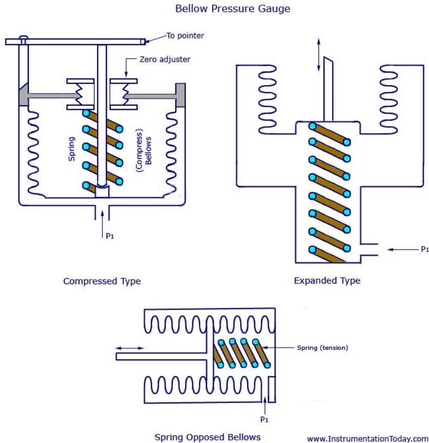
Fig. 1. Diagram of a Bellow Pressure Gauge<sup>1</sup>
