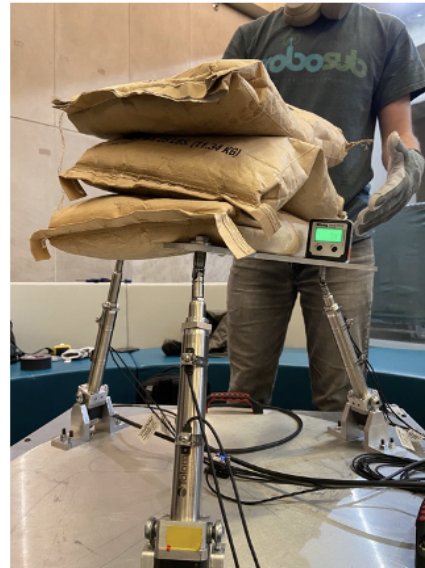
Figure 14: Dynamic load test of the leveling subsystem
